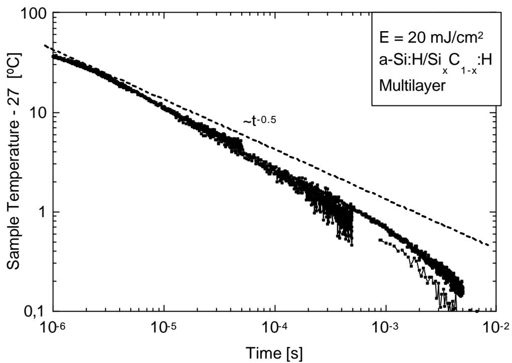
**Fig.5** (of 6) (a) Transient photoreflection for different laser beam intensities
