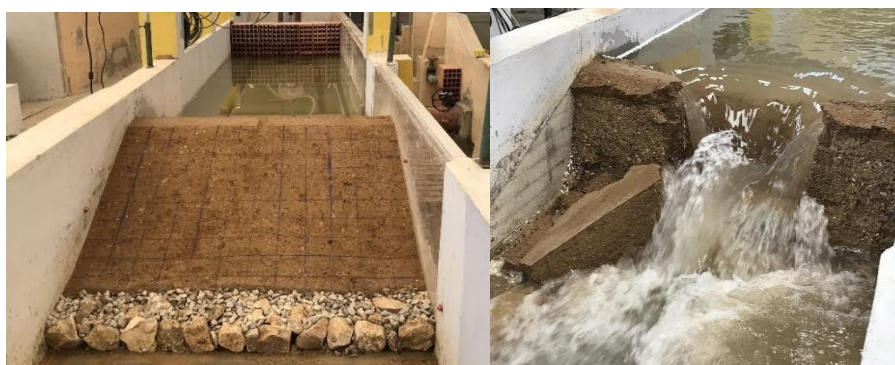
Figure 1. Left: example of physical model: 0.45 m tall embankment); right: erosion of an overtopped non-homogeneous embankment.
