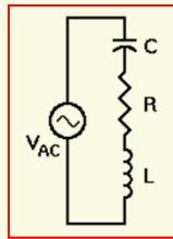
$$\langle P(\omega) \rangle = \frac{R\omega^2 \mathcal{E}_{ef}^2}{L^2(\omega^2 - \omega_0^2)^2 + R^2\omega^2}$$
