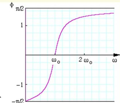
$$Z_{\text{series}} = \sqrt{R^2 + (\omega L - \frac{1}{\omega C})^2} \quad \phi = \tan^{-1} \frac{\omega L - 1/\omega C}{R}$$
